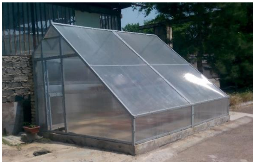
Figure 1. Solar dryer greenhouse device overview
